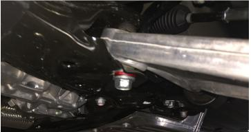
Pry down on the lower control arm to re-install the lower ball joint in the knuckle. Torque the lower ball joint nut to 65 ft-lbs and re-install safety hardware. Re-install the outer tie rod end, torque to 65 ft-lbs, and re-install safety hardware. Re-install brake rotor and caliper bracket. Torque caliper bolts to 100 ft-lbs. Re-attach ABS sensor and brake hose bracket. Torque bolts to 5 ft-lbs.
