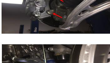
Remove the 4 bolts holding the gravel guard to the gravel guard to the suspension cradle and allow the guard to hang.
