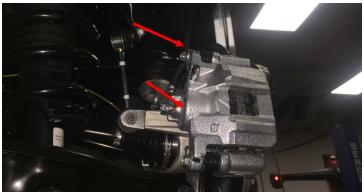
Loosen the nut holding the toe adjuster and the nut on the same arm at the hub. Loosen the 2 bolts holding the lower trailing arm.
