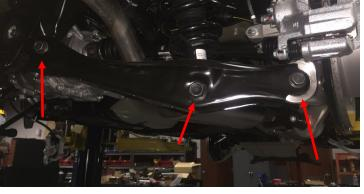
Remove 1 bolt at a time. Install spacers (shown in red) between the cradle and the body, and between the support brackets and the body. Use the provided M12 bolts for the bracket spacer.
