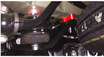
Raise the strut up with ReadyLIFT rear strut spacer (shown in red) and thread provided M12 bolts through. Do not tighten at this time.
