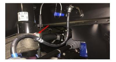
Remove the brake caliper bracket and support using a suitable hanger to prevent straining the rubber brake hose.
