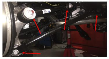
Remove the lower strut bolt. Loosen the control arm bolt at the cradle. Remove the control arm bolt at the hub and let the control arm swing out of the way.
