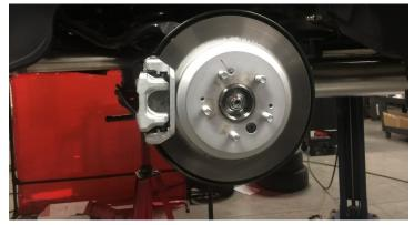
Remove the ABS sensor and brake hose bracket.
