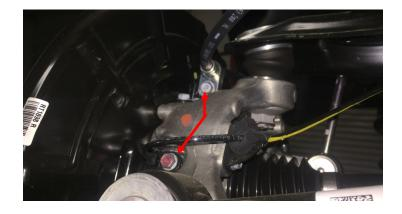
Un-bolt the sway bar end links at the knuckle. You may do this on both sides to facilitate movement.
