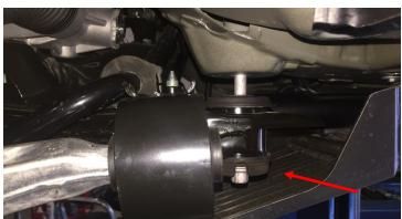
Remove the bolts holding the lower control arm to the cradle, and remove the lower control arm.
