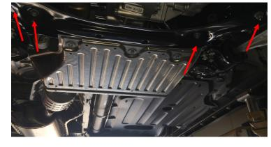
Loosen the front cradle to facilitate control arm removal and re-installation. There are 8 cradle bolts, 6 in front of the wheel hub, and 2 are behind the wheel hub. This step should be performed with the cradle supported safely. Do not remove cradle bolts or the cradle.
