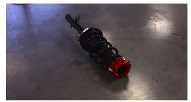
Raise the assembled strut into the vehicle and secure using provided hardware. Do not tighten at this time.
